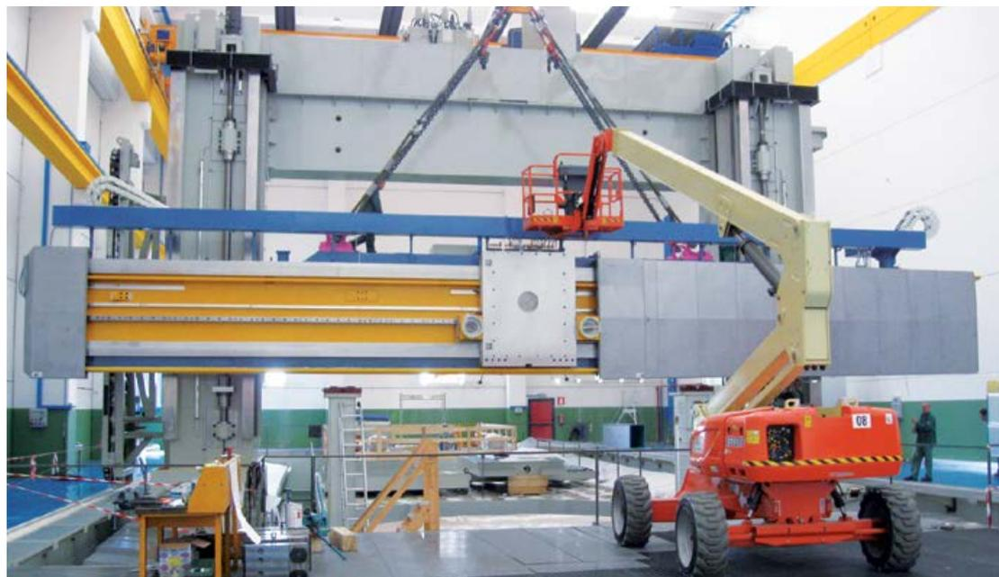
UNIMILL machines allow operation with pendulum concept: it is possible to have 2 separate areas on the floor table. One machining area, with protections and movable enclosures (optional) and one area to set up the part, that is accessible by means of bridge on the guideways covers.
